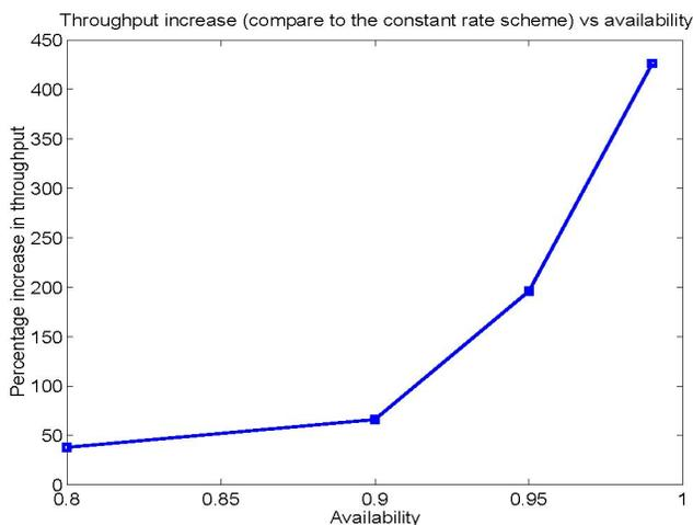
Fig. 1. Percentage throughput increase of ART scheme over CRT scheme for different link availabilities.
