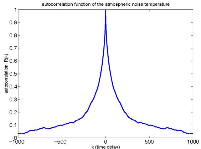
Fig. 3. The autocorrelation function of the atmospheric noise temperature data with sampling interval of 5 minutes.
