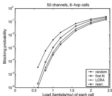
Fig. 10. Line network with 6-hop calls (length 6 units).
