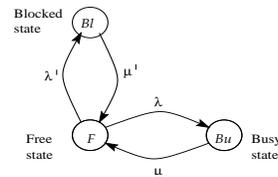
Fig. 3. Three state Markov process model of a channel on a link.
