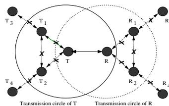
Fig. 1. Interference model for a bi-directional transmission ( $T \leftrightarrow R$ ).
