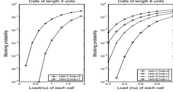
Fig. 6. Line network with calls of length 3 and 6 and 20 channels.
