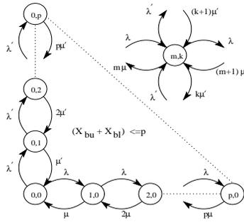
Fig. 4. State transition diagram for the random assignment policy.
