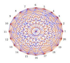
Figure 3: A network  $\mathcal{G}$  with N = 20 nodes. The colors of the edges indicate their directions (e.g., *blue edge*  $\implies$  $i \rightarrow j : i > j$  and vice versa). The broadcast capacity  $\lambda^*$ of the network is computed to be 6, with node 1 being the source node.
