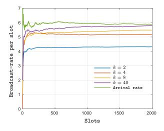
Figure 4: Achievable broadcast-rate with the multi-class heuristic broadcast-policies  $\pi_k^H$ , for k = 2, 4, 8, 40. The underlying network-topology is given in Figure 3.
