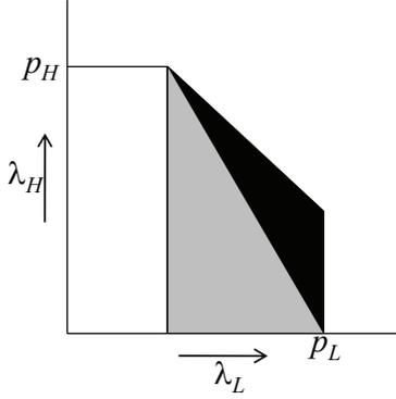
Fig. 4. Under max-weight- $\alpha$  scheduling with  $\alpha_L < \alpha_H$ ,  $q_L$  is light-tailed for arrival rates in the unshaded region, and heavy-tailed with tail coefficient equal to  $C_H - 1$  in for arrival rates in the gray region. For arrival rates in the region colored black, the tail coefficient lies in  $[\gamma, C_H - 1]$ .
