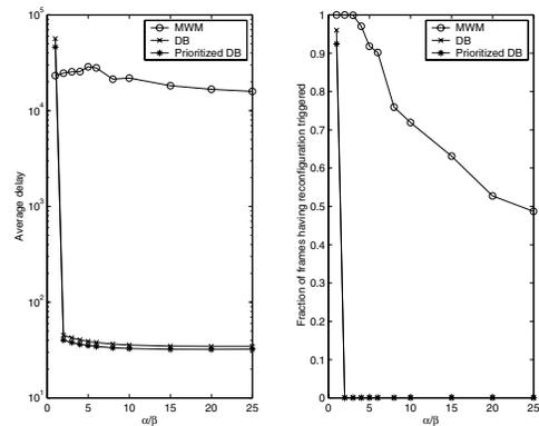
Fig. 11. Average delay (left) and fraction of frames in which a reconfiguration was initiated (right) for a range of  $\alpha/\beta$  values.  $N = 6$  nodes,  $D = 1000$  time slots. Each non-hub node has an average arrival rate of  $\alpha + (N - 2)\beta = 0.9$  packets per slot.
