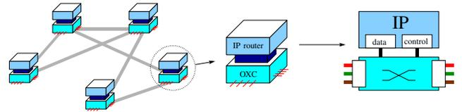
(a) IP-over-WDM network architecture, with each node consisting of an optical crossconnect and an IP router. The network at the left is a 5-node physical topology.
