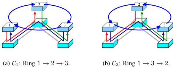
Fig. 2. Lightpath interconnections for 3-node rings on a line physical topology.
