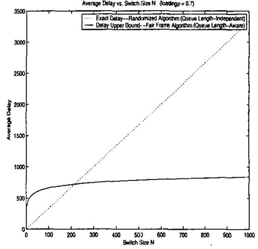
Fig. 2. The logarithmic delay bound for the Fair-Frame algorithm as a function of the switch size  $N$ , as compared to the  $O(N)$  delay of the randomized algorithm (which was previously the best known delay bound).
