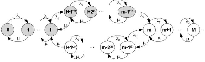
Fig. 2. The Markov process  $Y(t)$  corresponding to the two-threshold control policy.
