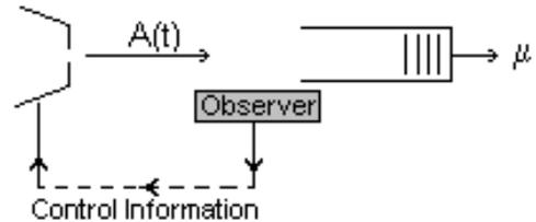
Fig. 1. A single server queue with input rate control.
