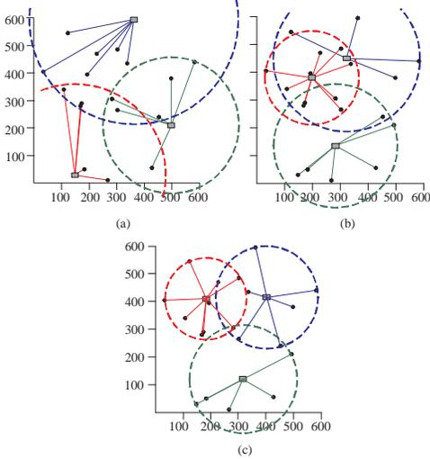
Fig. 7. Example of solutions found for a  $K = 3$ ,  $N = 20$  instance of the MFPA problem with the Slotted Aloha throughput function. (a) Unoptimized Farthest Point Heuristic (FPH) (b) Unoptimized Extended Diameter Algorithm (c) Optimal MFPA algorithm.
