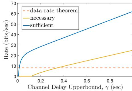
**Fig. 9** Sufficient and necessary transmission rates for stabilization. Here we have a scalar system with disturbances bounded by 0.4, with  $A = 5.5651$ . The rate dictated by the data-rate theorem is  $R_c \geq A/\ln 2 = 8.02874$ .
