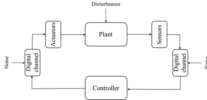
**Fig. 1** High level abstraction of a CPS from a communication perspective.
