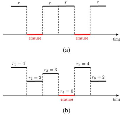
**Fig. 5** Example of stochastic channels. (a)  $r$ -bit packet erasure channel. (b) stochastic-rate channel, including erasures.
