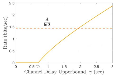
**Fig. 8** Phase transition of the necessary information transmission rate for stabilization. The graph is valid for any generic system. In this example we have a scalar system with no disturbance,  $A = 1$ ,  $\gamma_c = \ln 2/A = 0.6931$  and the rate dictated by the data-rate theorem is  $R_c \geq A/\ln 2 = 1.4427$ .
