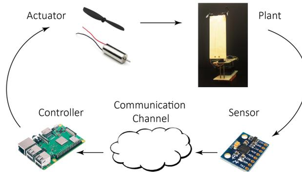
**Fig. 12** Architecture and components of the prototype.
