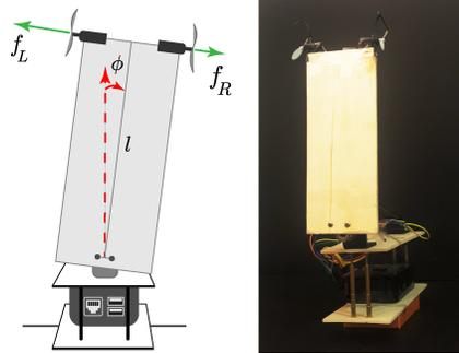
**Fig. 11** An inverted pendulum controlled by thrust force of two propellers. The angle  $\phi$  of the pendulum from the vertical line and its rate of change, measured by the sensor and transmitted to the controller over a digital channel with bounded unknown delay, are used to determine the left and right thrust forces of the propellers.
