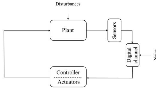
**Fig. 2** Simplified model where the controller is co-located with the actuators.
