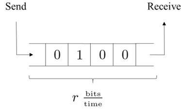
**Fig. 4** Bit-pipe channel
