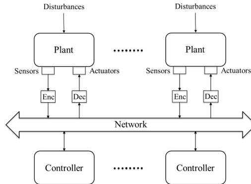
**Fig. 3** Distributed communication and control system.
