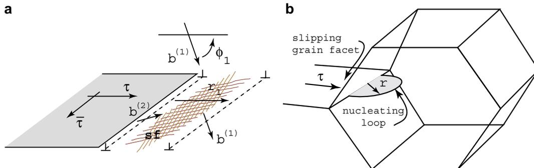
Fig. 11. (a) A model for partial dislocation emission from a grain boundary that acts in a crack-like manner. The crack is loaded via an in-plane Mode II applied stress,  $\tau$ , and an anti-plane Mode III shear stress,  $\bar{\tau}$ . (b) Nucleation of a partial dislocation loop at the front of a freely slipping grain boundary facet. (Figure taken from Ref. [127].)
