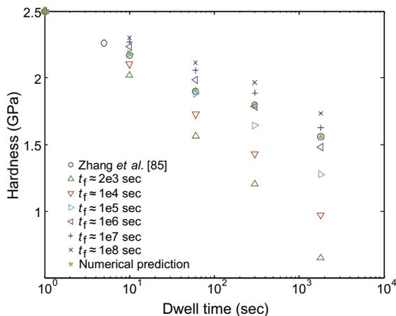
Fig. 13. Simulated hardness vs. time [93], compared with the measurements of Zhang et al. [85]. The simulations were performed using a wide range for  $t_f$ , i.e.  $2 \times 10^3 \text{ s} \leq t_f \leq 10^8 \text{ s}$ . (Figure taken from Ref. [93].)
