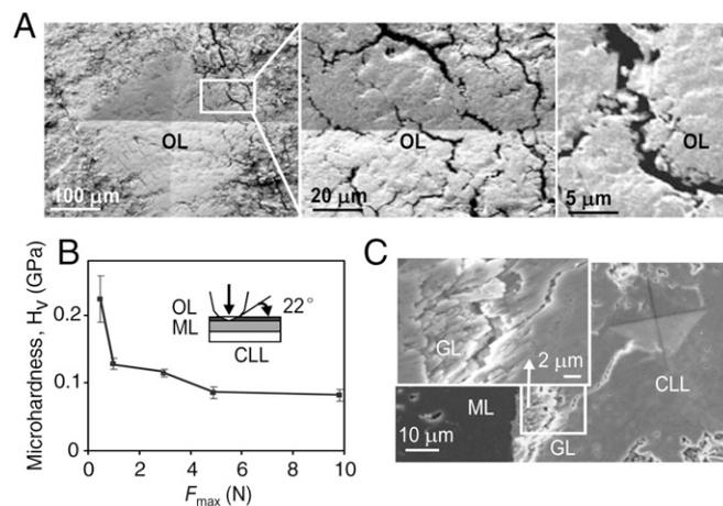
**Fig. 4.** Microindentation of the shell of *C. squamiferum*. (A) SEM images of residual indents of Vickers microhardness experiments with load normal to the shell surface (maximum load approximately 9.8 N, depth 62  $\mu\text{m}$ ). (B) Measured Vickers hardness as a function of the maximum applied load (error bars indicate standard deviation). (C) SEM images of residual indent (load applied normal to cross section of GL). *Inset* shows the fracture processes in the GL.
