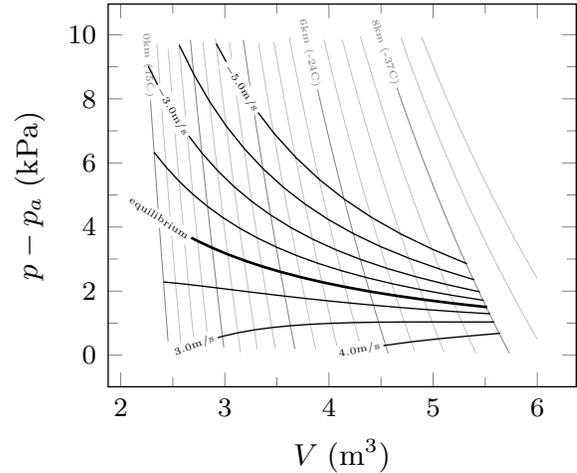
**Figure 2: Pressure-volume diagram for a constant-mass (3 kg) balloon in thermal equilibrium with a standard atmosphere. See text for explanation.**
