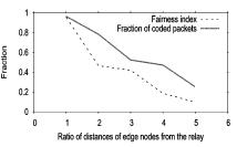
Fig. 14. Effect of unequal channel qualities on coding opportunities and throughput gain in the Alice-and-Bob topology. COPE aligns the fairness and efficiency objectives. Increased fairness increases coding opportunities and hence improves the aggregate throughput.
