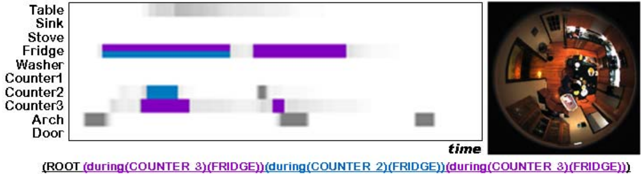
Figure 5. Significant patterns are matched in multi-variate time series representations of events. These patterns are collected together under a dummy root node for use with a tree kernel based Support Vector Machine. Single patterns can be instantiated multiple times in an event and individual events can participate in multiple patterns.
