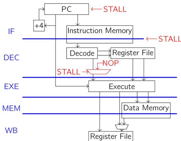
When **STALL** is 1, the PC doesn't accept a new value, and the IF stage will also keep operating on the same instruction it's been working on (meaning the Decode stage will also still see the same inputs from the previous cycle).
