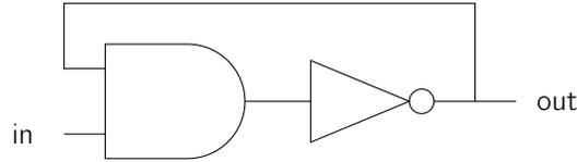
This circuit contains an AND gate and an inverter (we can tell the difference between an inverter and a buffer by the circle at the tip). The point is that if our input bit is 1, our circuit will not settle at a particular output value (or voltage), meaning there is no well-defined propagation delay.
