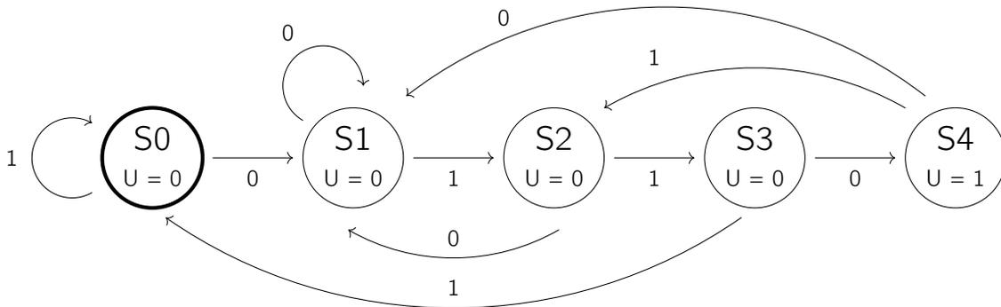
We give each state a name (**S0** through **S4**), and each state has an associated output. (In this case, only being in **S4** will allow us to unlock the lock.) We put a heavy circle around the initial state to indicate that it is where we
