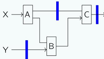
The issue with this circuit is that the path through A and C starting from X, as well as the path through B and C starting from Y, each go through 2 registers. But the A-B-C path only has a single register, so that's going to **mix our calculations together between cycles!** Specifically, we're looking at  $A(X_{i+1})$  and  $Y_i$  being fed into B at the same time; that's the kind of thing that we need to be careful about.
