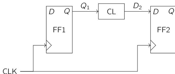
Then we need to make sure that the input  $D_2$  is stable at least  $t_{\text{SETUP}}$  before the next rising edge of the clock, but before that can happen, we need our bit  $D$  to propagate through our first flip flop FF1, which then goes through the combinational logic. So we need at least  $t_{\text{PD, FF1}}$  from the first flip flop, plus some time  $t_{\text{PD, CL}}$  to turn a stable  $Q_1$  into a stable  $D_2$ , to all happen early enough. In other words, we need the inequality
