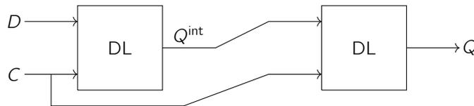
Here, we’re using the same control signal  $C$  for both latches, so they’ll both pass at the same time and also hold at the same time. So having two of these in series doesn’t do anything for us. But we can also combine these two D latches in a different way: **for one of the D latches, we feed in the negative of the control signal**, and we can do this by **adding an inverter to the bottom C path**.
