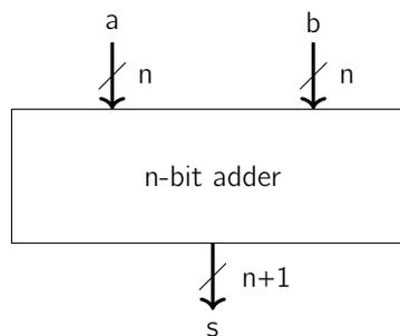
(Remember that  $n$  must be fixed in any particular circuit, though – it's not an input.) The way we'll implement this is by using the **standard addition algorithm** we use normally: start adding from the least significant bits and carry a 1 to the next column if necessary. This is better than starting from the truth table, since such a table for a 32-bit adder would give us  $2^{64}$  different rows (which is definitely impossible in practice).
