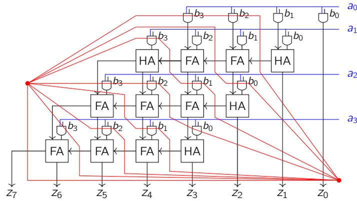
In each pipeline stage, we only have one full adder worth of delay now, meaning that our  $t_{CLK}$  is  $\Theta(1)$  (it's just the amount of time through a single full adder), and we have  $\Theta(N)$  different pipeline stages. So the latency remains  $\Theta(N)$ , but we've **improved our throughput** to  $\Theta(1)$ , which is significantly better. (In words, once we've filled our pipeline, we're able to produce a new valid output once per cycle!)
