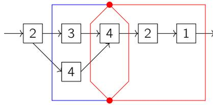
But the red contours don't exactly finish the job for us – the clock time is still greater than 4 ns, unless we add the blue pipeline stage to split up the  $2 + 3 = 5$  ns delay from the top two circuit components. This gives us  $t_{CLK} = 4$ , so  $L = 16$  and  $T = \frac{1}{4}$ .
