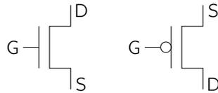
In other words, feeding a 1 into the nFET on the left gives us a path from D to S, while a 0 leaves the circuit closed. But feeding a 0 into the pFET gives us a path, while a 1 does not.
