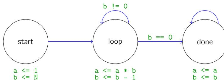
So at each cycle, we're in one of these three states, and we transition between states and do operations based on the values stored in our registers.
