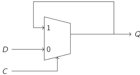
In this circuit, we still have a feedback path that maintains the current state, but we also have a new way to load a value. The multiplexer has an output tied to one of its inputs – if the control signal is 1, then we’re using the feedback path where we maintain the old value, so  $Q$  holds at its current value. On the other hand, if the control signal  $C$  is 0, then we select the input  $D$ , and we can propagate the new value.
