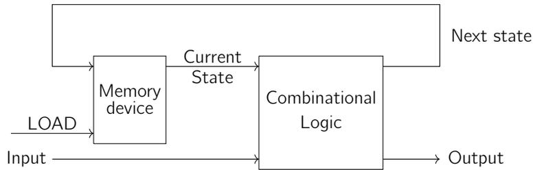
Here, the memory device stores our current state, and the combinational logic device computes two things:
