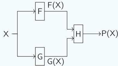
This circuit has three submodules  $F, G, H$ , and the latency of this circuit, also known as the propagation delay, is the sum of the times along the slowest path in the circuit. So if we have a latency of  $t_{PD}$ , then the combinational throughput will be  $\frac{1}{t_{PD}}$  (that's how many outputs per second we can produce).
