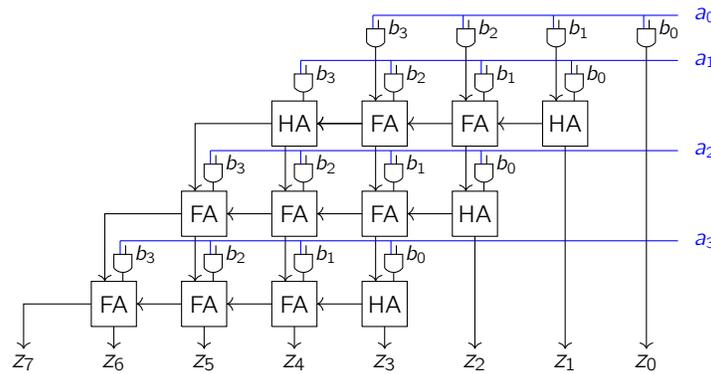
Right now, our latency is of order  $N$  for an  $N$ -bit adder, because the longest path in the circuit goes across a full ripple-carry adder and also goes down through the various levels, giving us about  $2N$  gates. So using a combinational  $N$ -bit multiplier gives us a latency of  $\Theta(N)$  and a throughput of  $\Theta(1/N)$ . (And we can also check that our area is  $\Theta(N^2)$ .)
