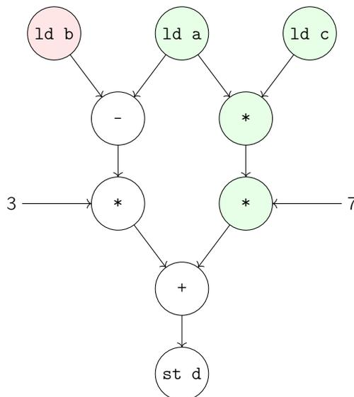
The arrows represent outputs and inputs for each of the operations, and indeed we can see that there are parts of the dataflow that don't depend on others. So modern processors use this kind of internal representation to see which
