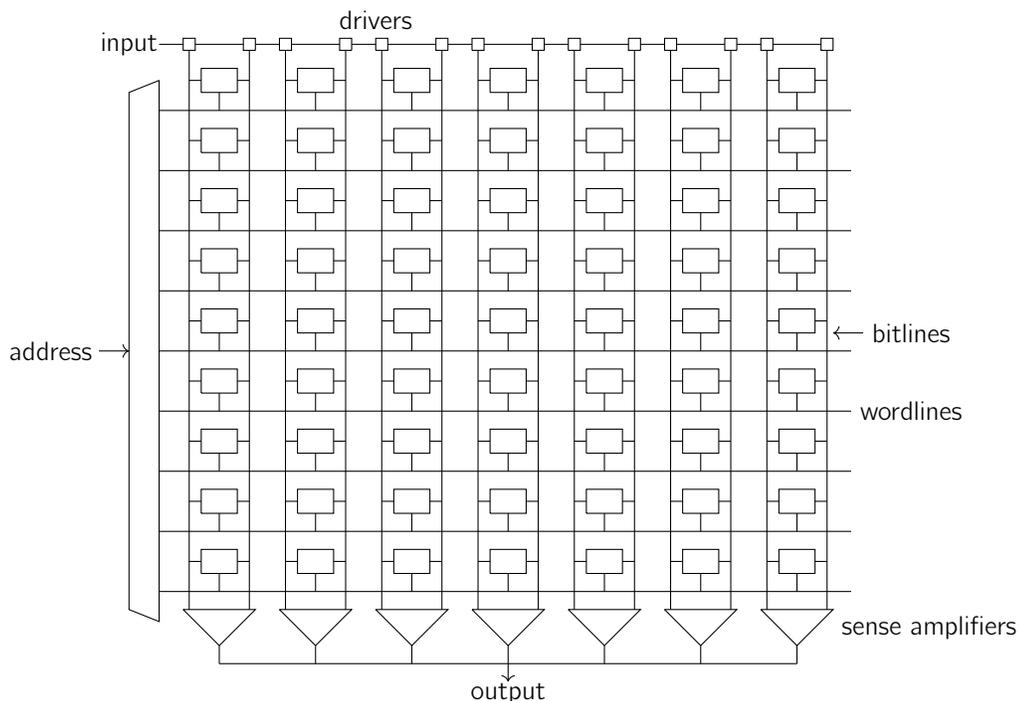
Data comes out of one end of the SRAM. At the output end of each vertical bitline, we have **sense amplifiers**, helping to detect small changes and amplifying them so that outputs are provided more quickly. Finally, data is fed in through inputs from the **drivers** (on the opposite side of the sense amplifiers), and we can write to our SRAM by setting bitlines to appropriate voltages.
