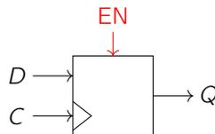
We’ve added one more input here, called an **enable signal**, and the idea is that we only capture new data  $D$  if the enable bit  $EN$  is equal to 1. We implement this by **putting a multiplexer in front of our D flip flop** – the circuit says that if the  $EN$  bit is 0, we keep our old state, and otherwise, we accept a new value of  $D$  to propagate over to  $Q$ . So when the enable bit is 0, we hold, and when the enable bit is 1, we copy the input.
