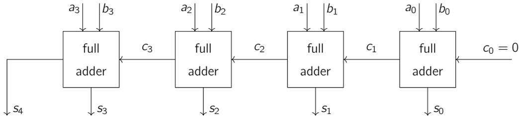
This is called a **ripple-carry adder** – it's simple and it's the cheapest adder in terms of area, but it's **slow** because of the series connections, and thus the propagation delay adds up across the  $n$  full adders. We'll see how to optimize this (to scale as  $\log n$  instead of  $n$ ) soon, but for now let's go back to the (one-bit) full adder and understand it more clearly.
