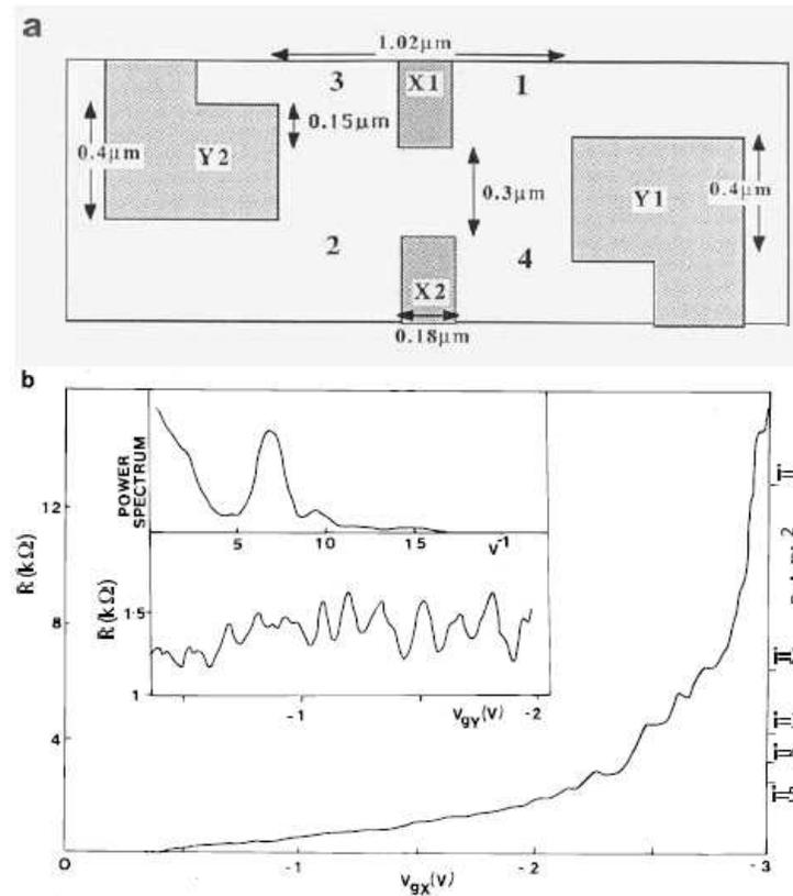
(a) Schematic diagram of a constriction with two adjustable external reflectors defined by gates on top of a GaAs-AlGaAs heterostructure. (b) Plot of the constriction resistance as a function of gate voltage with the external reflector gates (Y1, Y2) grounded. Inset: Fabry-Perot-type transmission resonances due to a variation of the gate voltage on the reflectors (Y1, Y2) (bottom panel), and Fourier power spectrum (top panel). Taken from C. G. Smith et al., *Surf. Sci.* **228**, 387 (1990).
