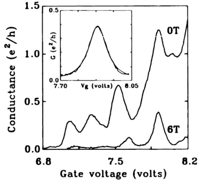
Oscillations in the conductance as a function of gate voltage at 0.5 K are attributed to resonant tunneling through localized states in the potential barrier. A second trace is shown for a magnetic field of 6 T (with a horizontal offset of  $-0.04\text{V}$ ). The inset is a close-up of the largest peak at 6 T, together with a Lorentzian fit. Taken from T. E. Kopley et al. Phys. Rev. Lett. **61**, 1654 (1988).
