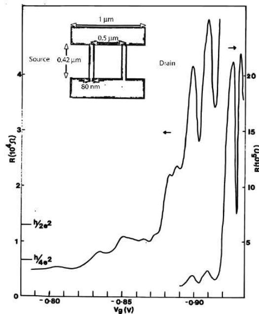
Resistance versus gate voltage of a cavity (defined by gates on top of a GaAs-AlGaAs heterostructure; see inset), showing plateau like features (for  $R \lesssim h/2e^2$ ) and tunneling resonances (for  $R \gtrsim h/2e^2$ ). The left- and right-hand curves refer to the adjacent resistance scales. Taken from C. G. Smith et al., Surf. Sci. **228**, 387 (1990).
