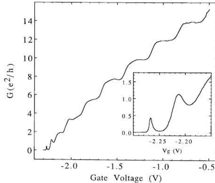
Conductance as a function of gate voltage for a quantum point contact at 0.55 K. The inset is a close-up of the low-conductance regime, showing peaks attributed to transmission resonances associated with impurity states in the constriction. Taken from P. L. McEuen et al., *Surf. Sci.* **229**, 312 (1990).
