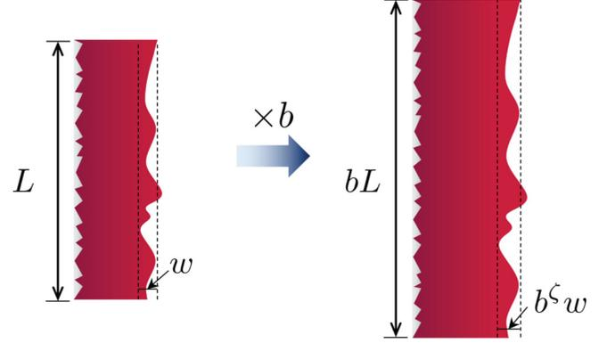
FIG. 8. An illustration of the scaling procedure used to construct the Imry-Ma argument. As the system size is increased by a factor of  $b$ , the width of the interface between the phases is multiplied by  $b^\zeta$ . The interface is well defined in the large system-size limit when  $\zeta < 1$ .
