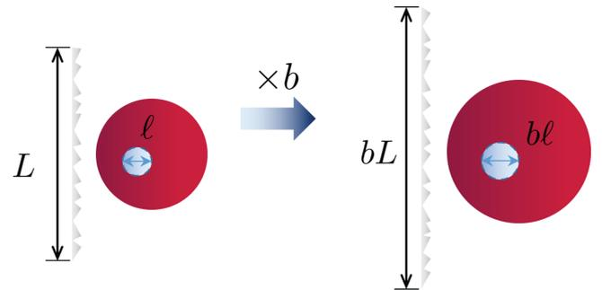
FIG. 11. The scaling argument presented in Fig. 9 for the wetting layer can be adapted to the case of a liquid droplet. Upon scaling the system size by a factor of  $b$ , we compare the scaling of the bulk and surface energies, whose competition determines if the droplet is macroscopically stable.
