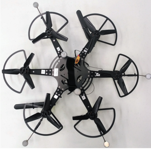
Fig. 7: Custom hexarotor used in the hardware experiments. It is equipped with the Qualcomm ® Snapdragon Flight, which is where the controller and the observer run.
