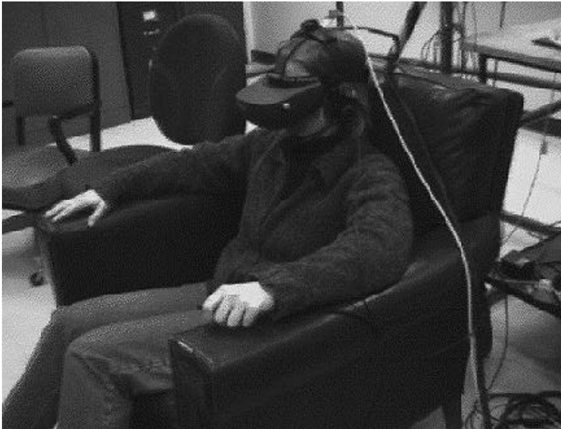
Figure 3.19: The experiment station. A subject sits comfortably, wearing the HMD and holding the "push to talk" button for the voice recognition system.
