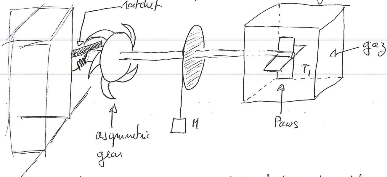
Idee: The gear can easily rotate clockwise but the ratchet prevents counter-clockwise rotations. Fluctuations of the paws are thus rectified and the gear rotates in one direction, lifting the mass  $M \rightarrow$  motor.
