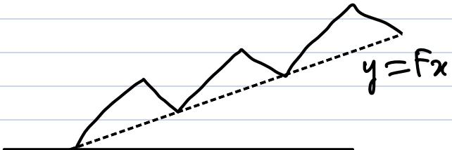
$$\text{Energy barrier } \Delta E: \text{forward rate } p = p_0 e^{-\beta \Delta E} \Rightarrow p_1 = p_0 e^{-\beta [\Delta E + F(l-\delta)]}$$
