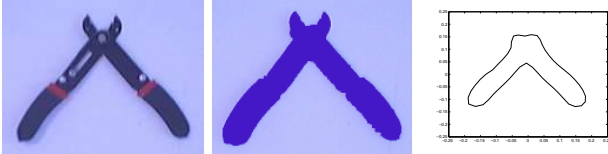
Figure 3. Full-contour shape representation. Left to right: original image, an example extracted contour and the mean of the learned shape class. The top of the tool is slightly rounded off due both to the small number of points (50) sampled from the contour to form the preshape, as well as to the smoothing effect of computing the mean shape of the tool as it opens and closes.
