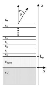
FIG. 1. Cross-sectional view of vertical-cavity enhanced resonant thermal emitter (VERTE).
