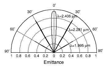
FIG. 7. Polar plot of silver-VERTE emittance (for TE polarization) at three different wavelengths (2.406, 2.281, and 1.995  $\mu$ m) corresponding to resonant peak maximums at  $\theta$  of 0°, 30°(TE polarized), and 60°(TE polarized).
