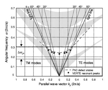
FIG. 2. Projected band diagram of 1D photonic crystal with a defect state and VERTE projected resonant modes.
