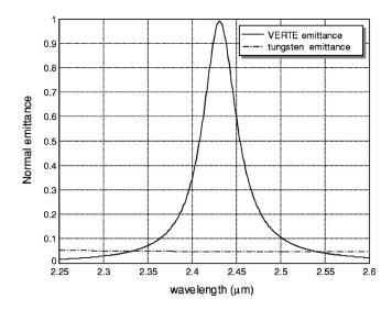
FIG. 3. Normal emittance of vertical-cavity enhanced resonant thermal emitter with tungsten and normal emittance of planar tungsten.
