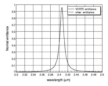
FIG. 4. Normal emittance of vertical-cavity enhanced resonant thermal emitter with silver and normal emittance of planar silver.
