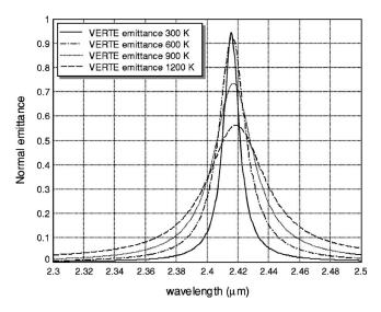
FIG. 8. Normal emittance of VERTE structure  $[(LH)^3L^2$ -silver] for 300, 600, 900, and 1200 K.
