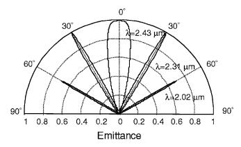
FIG. 6. Polar plot of tungsten-VERTE emittance (for TE polarization) at three different wavelengths (2.43, 2.31, and 2.02  $\mu$ m) corresponding to resonant peak maximums at  $\theta$  of 0°, 30°(TE), and 60°(TE). Directional resonant emittance peaks are also designated in Fig. 2 as squares.
