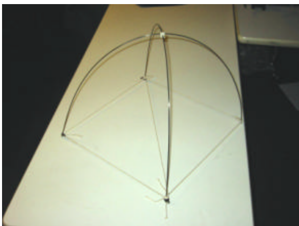
Figure 2 Frame structure of the tent showing the carbon fiber rods held together by string
