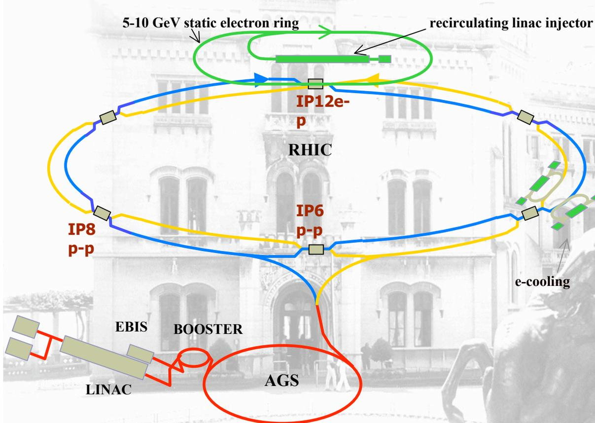
Linac injects into electron storage ring at full energy
