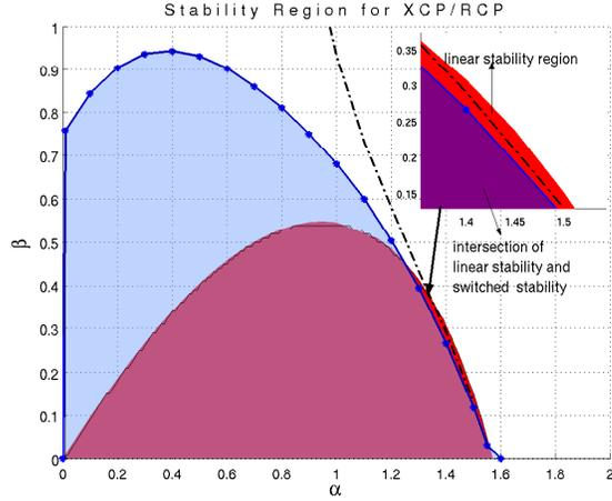
Fig. 6. Provably safe regions of  $\alpha$  and  $\beta$  (for  $d = 200$  ms)
