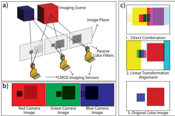
**Figure 3: Trinocular Lensing System.** a) shows the three CMOS imaging sensors equipped with passive color filters imaging two cubes. The camera viewpoint can be seen on the imaging plane. b) shows the images captured from the three monochrome cameras equipped with color filters. c) shows the results of 1. Direct Combination, 2. Linear Transformation alignment and 3. Original Color Image if captured from a color camera
