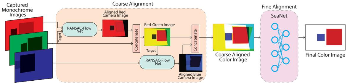
**Figure 4: Cross Color Alignment:** works in two steps 1) Coarse Alignment and 2) Fine Alignment. In Coarse Alignment, RANSAC-Flow Net coarsely aligns the images in a pairwise fashion. This coarse aligned color image then goes through the Fine Alignment step where SeaNet produces the final color image
