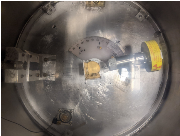
FIG. 2. A run at a \theta = 14.4^\circ scattering angle. The howitzer on the right is positioned to be in line with the gold foil target, and counts are recorded by the silicon barrier detector on the left.
