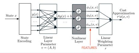
Given a set of state-cost training pairs  $(x^s, \beta^s)$ , s = 1, ..., q, the parameters of the neural network (A, b, r) are obtained by solving the training problem
