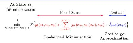
At state x<sub>k</sub>, we solve an ℓ-stage version of the DP problem with x<sub>k</sub> as the initial state and J<sub>k+ℓ</sub> as the terminal cost function
