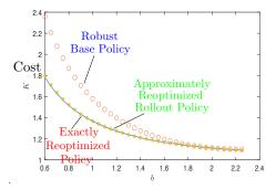
Performance comparison of on-line replanning by rollout and by optimization Note the effect of Newton's method
