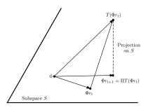
$$\Phi r_{t+1} = \Pi T(\Phi r_t)$$
