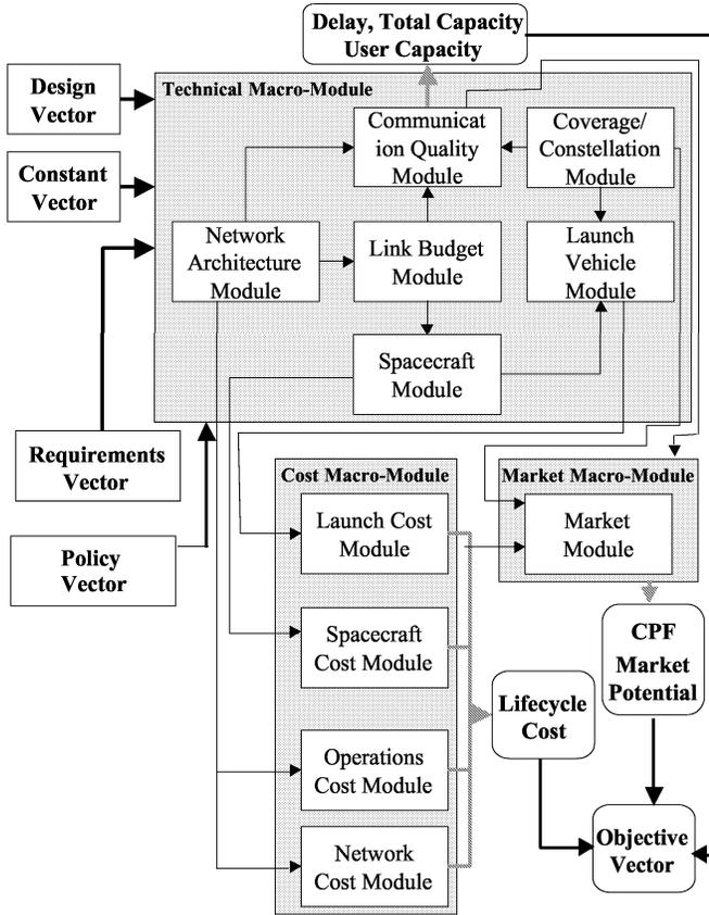
Fig. 5 LEO Communications Constellation Simulation Block Diagram
