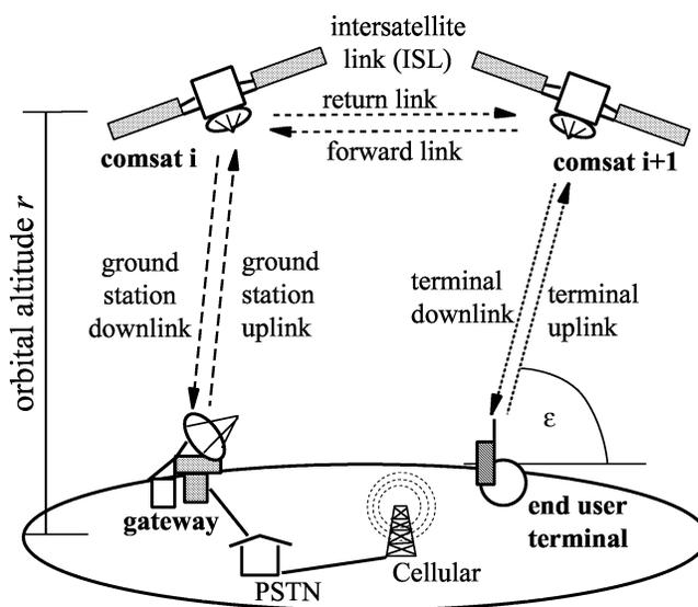
**Fig. 2 LEO Communication Constellation Architecture.** The end user terminal connects to a satellite *comsat i+1* via the terminal up/downlink when outside of cellular coverage. Voice and data is transferred to *comsat i* via intersatellite link. The downlink to a ground station (gateway) provides connectivity to the Public Switched Telephone Network (PSTN) and wireless cellular systems.
