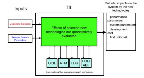
Figure 3-9: Technology infusion interface (TII) structure diagram
