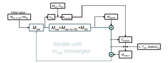
Figure A-7: Iterations to find satellite mass
