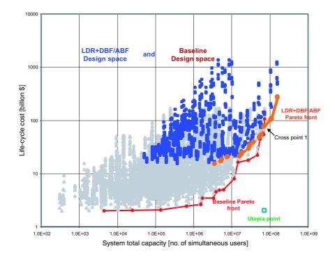
Figure 3-17: LDR+DBF/ABF-infused objective space and Pareto front
