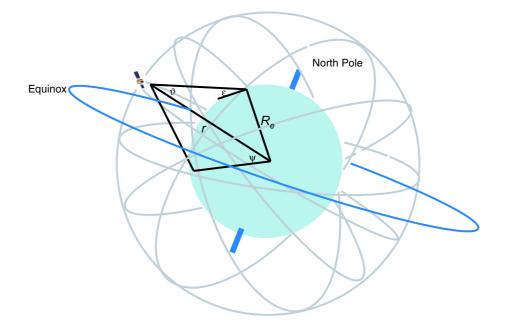
Figure A-3: Geometry of a Walker constellation
