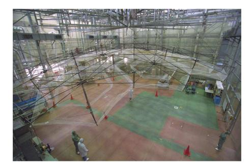
Figure 3-6: LDR engineering model deployment test (Copyright: NASDA)
