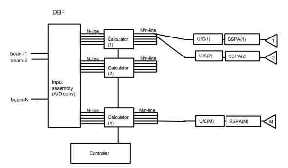
Figure D-1: Component diagram of DBF
