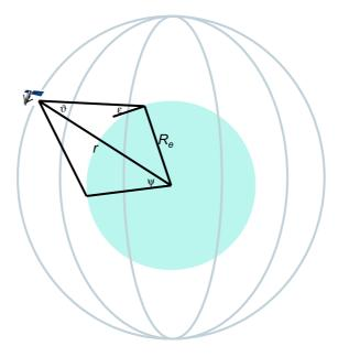
Figure A-2: Geometry of a polar constellation
