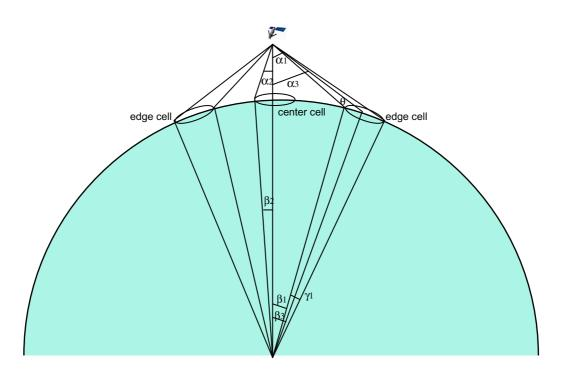
Figure A-4: Geometry involved in calculating single satellite coverage
