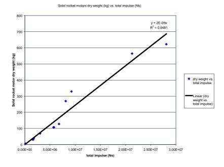
Figure A-8: Solid motor dry weight vs. total impulse
