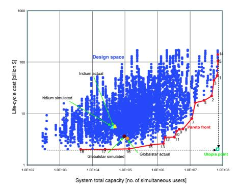
Figure 2-7: LCC vs. system capacity plot for a full-factorial run of 5,832 designs
