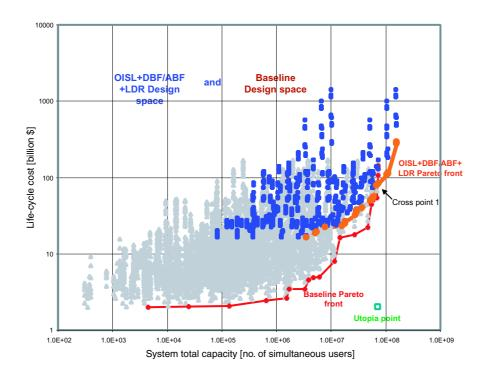
Figure 3-18: LDR+DBF/ABF+OISL-infused objective space and Pareto front
