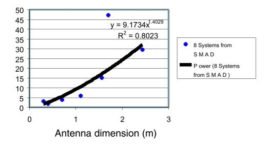
Antenna mass vs. antenna dimension for 8 system:
