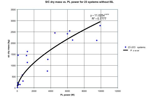
Figure A-5: Relationship between spacecraft dry mass and payload power for satellites with no ISL, based on the FCC filings of 23 LEO personal communication systems.
