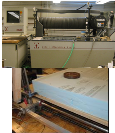
(b) Abrasive water-jet cutting machine and foam cutter machine
