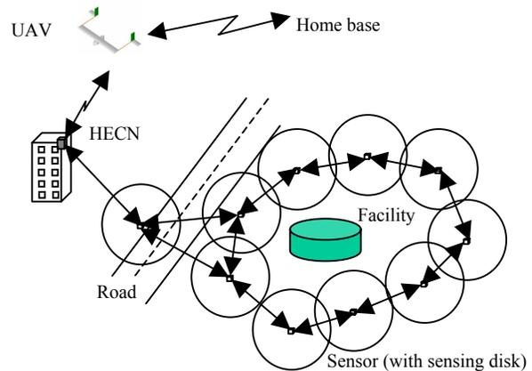
Fig. 1. Example of the use of a WSN to monitor a facility, with the High Energy Communication Node (HECN) placed on top of a building.
