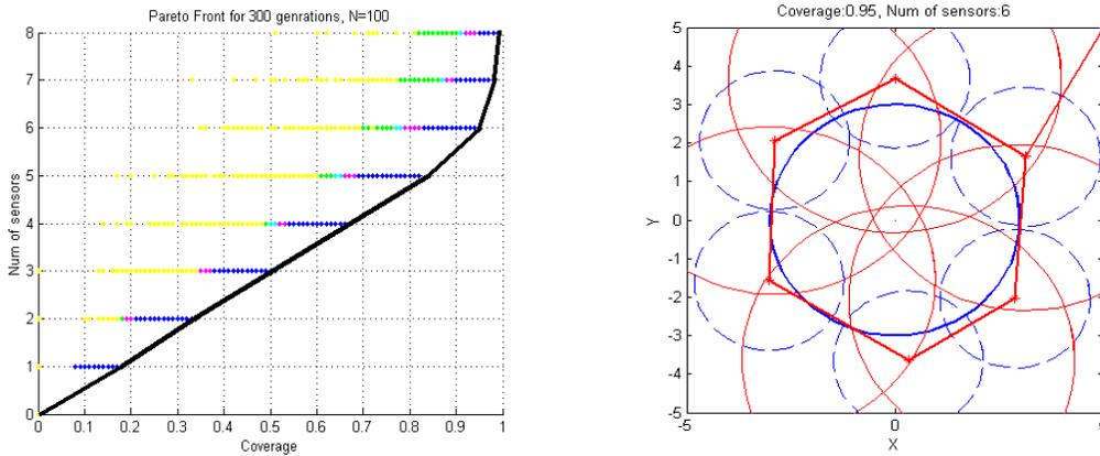
Fig. 7. MOGA results for Case 2: Objectives graph with Pareto Front (a, left) and WSN layout with 6 sensors (b, right)
