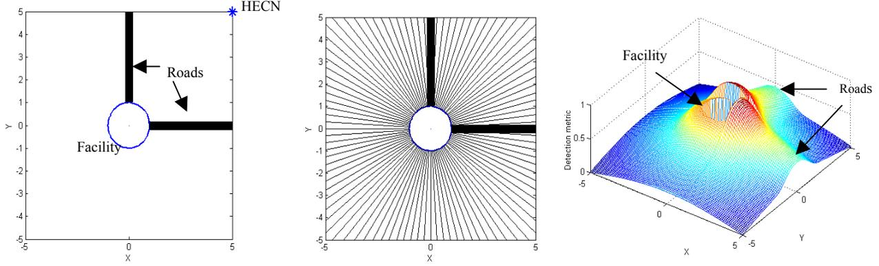
Fig. 2. Framework for Case 1: facility served by two roads (a, left); lines used to calculate the coverage objective (b, center); mapping of the probability of detection used for the survivability objective (c, right)
