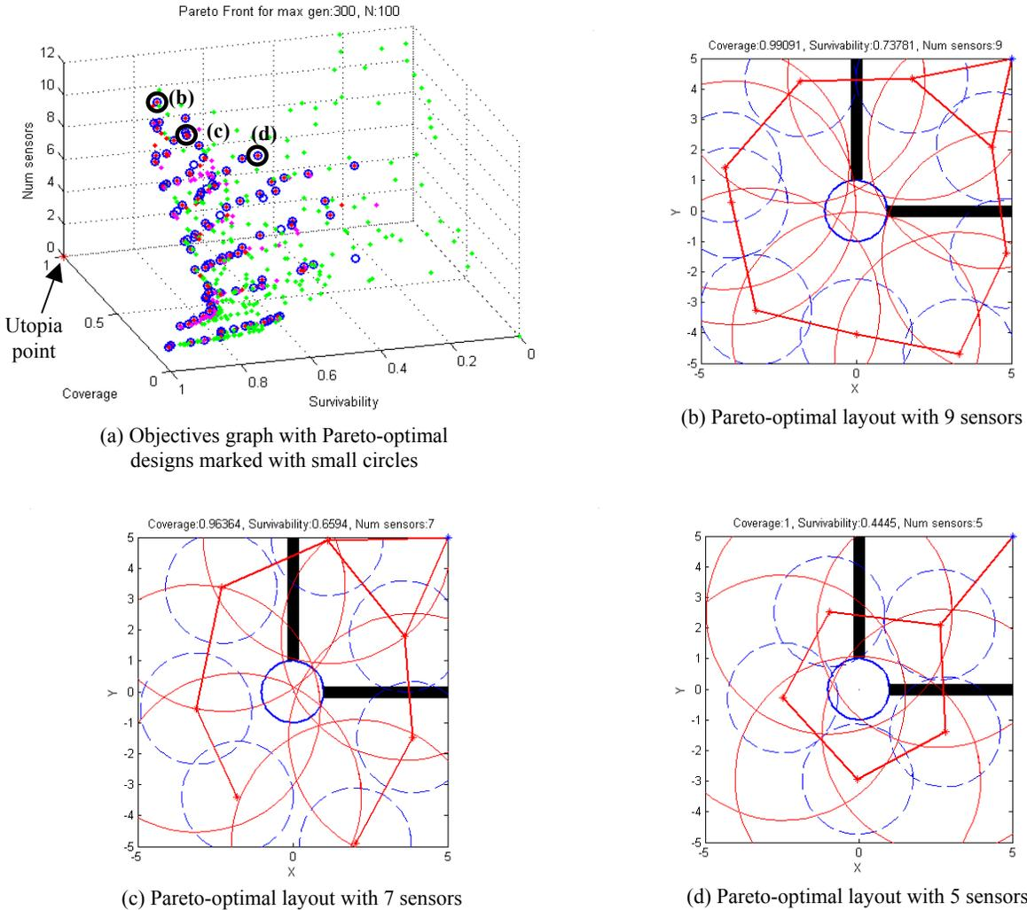
Fig. 6. MOGA results for Case 1. Objectives graph with Pareto Front and instances of Pareto-optimal WSN layouts (see legend of Fig. 4d)
