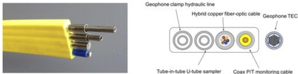
Figure 2 The MBM 'flatpack' (left) and the individual lines (right). Taken from (Daley *et al.* 2013b). The DAS data were recorded using one of the four fibres in the hybrid fibre-optic cable.
