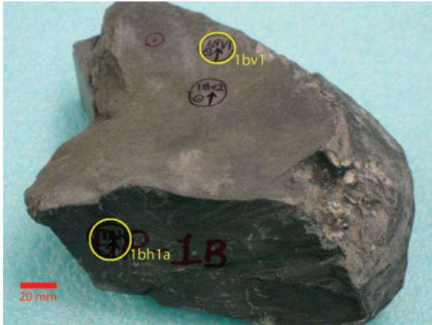
**Figure 1** Sample of the mudstone recovered from the exploration well. Marks indicate the location of the 20 mm plug samples cut parallel and perpendicular to the bedding.
