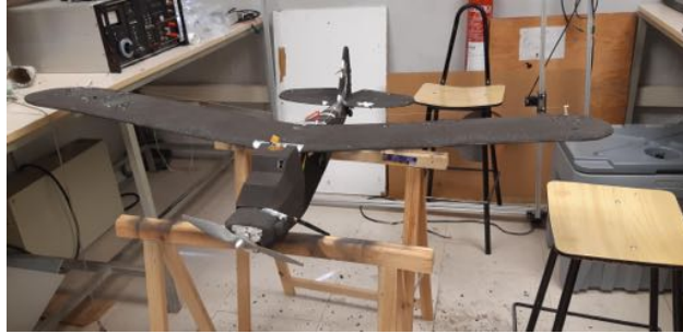
Fig. 8 RC aircraft fitted with corona wire along wingspan, pitot tube in vertical stabilizer, EFM mounted flush to the surface, and spray painted with conductive paint.
