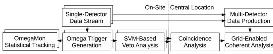
Fig. 2. Real-time GWB search pipeline.
