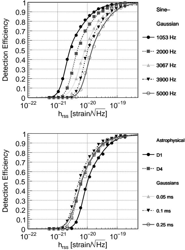
FIG. 5: Software injection efficiency curves for the set of sine-Gaussians of various frequencies (top) and Gaussians plus astrophysical waveforms (bottom). There is a consistent reduction in efficiency as a function of frequency following the noise distribution.
