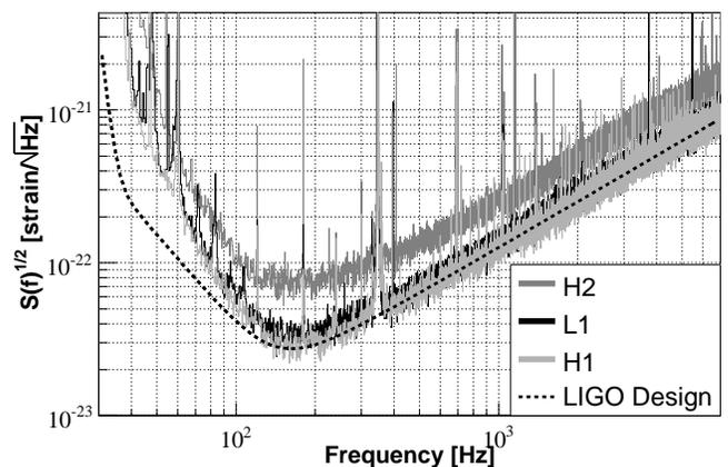
FIG. 1: Characteristic LIGO sensitivity curves from early in the S5 run. The sensitivity improved from February 2006 onward. Shot noise dominates the spectrum at high frequencies.
