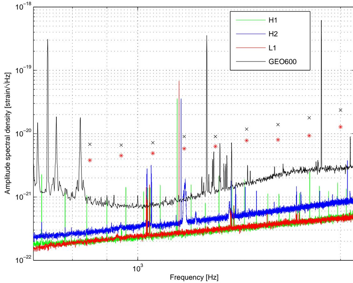
**Figure 8.** The  $h_{\text{rss}}^{50\%}$  values for Waveburst-CorrPower ('x' markers) and coherent Waveburst ('\*' markers) pipelines for sine-Gaussians of different central frequencies. Coherent Waveburst is sensitive to gravitational wave signals with amplitudes 30 – 50% lower than those detectable by Waveburst-CorrPower.
