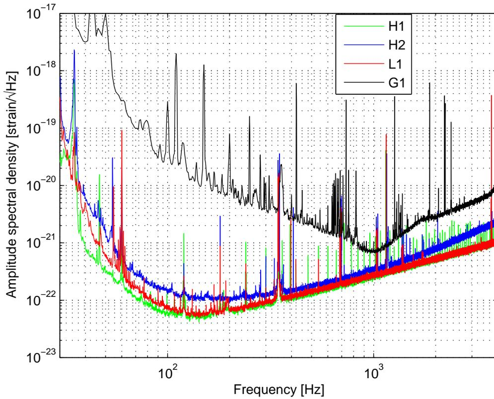
**Figure 2.** Strain spectral densities of the LIGO Hanford 2-km and 4-km detectors (H1, H2) and the LIGO Livingston detector (L1) as well as the GEO 600 detector (G1) during the S4 run. The plotted strain sensitivity curves are the best for the LIGO detectors, obtained on the 26th of February, 2005, for H1 and H2 and the 11th of March, 2005, for L1. The GEO 600 sensitivity curve is typical of the detector's performance during the S4 run.
