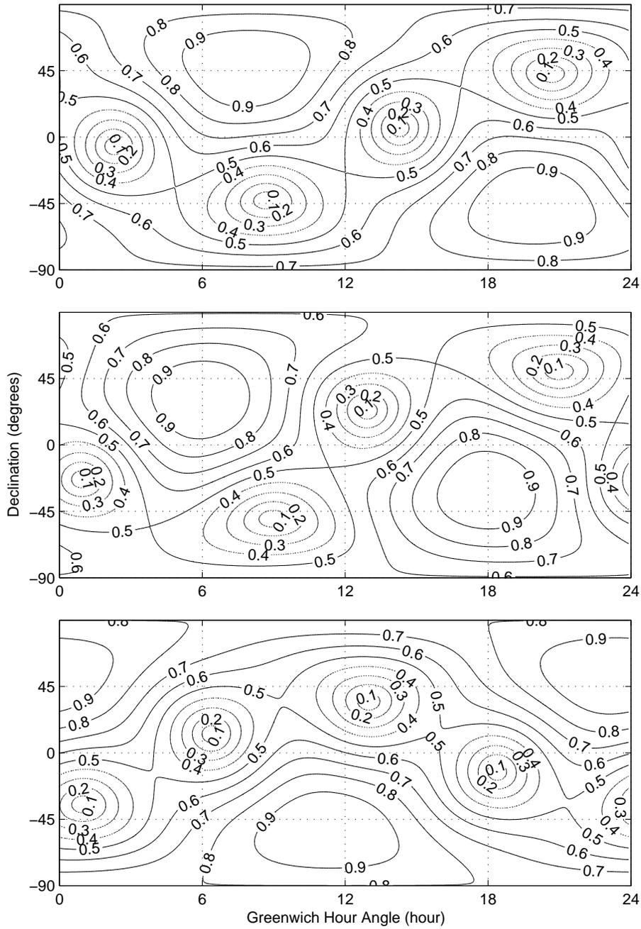
**Figure 1.** Antenna patterns ( $F_+^2 + F_\times^2$ ) of the Hanford (top), Livingston (middle) and GEO 600 (bottom) detectors. The locations of the maxima and minima in the antenna patterns for Hanford and Livingston are close. However, the antenna pattern for GEO 600 is different from those of the LIGO detectors.
