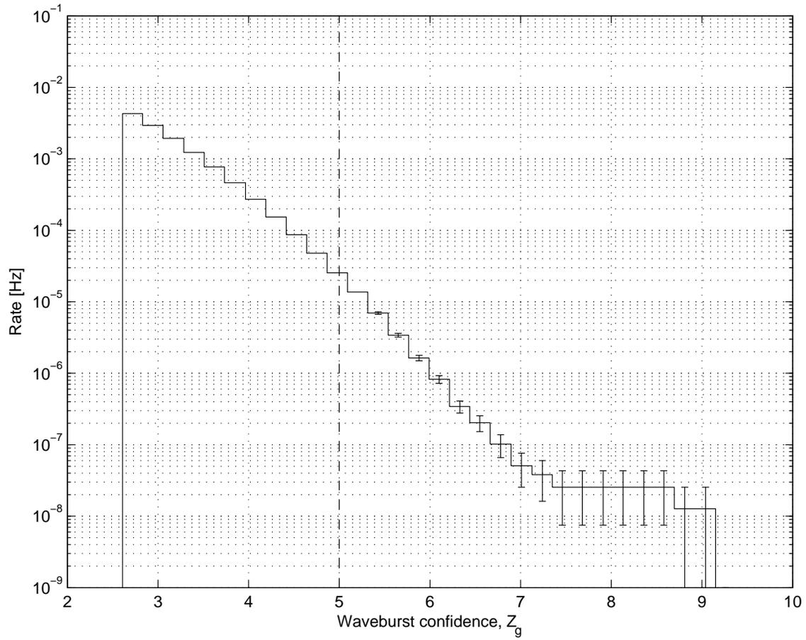
**Figure 3.** Quadruple coincidence rate as a function of the threshold on the Waveburst significance,  $Z_g$ . The threshold used for this analysis is indicated by the dashed line. The error bars indicate the range corresponding to  $\pm\sqrt{n}/T$ , where  $n$  is the number of triggers observed above the  $Z_g$  threshold over the livetime  $T$ .
