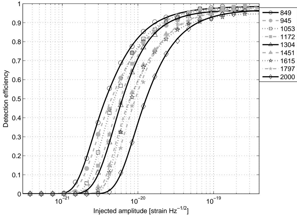
**Figure 7.** Detection efficiency of the coherent Waveburst pipeline for various sine-Gaussian simulated gravitational-wave bursts, as a function of the signal amplitude (defined by Eq. 18). The legend indicates the central frequency (Hz) of the injected signal.
