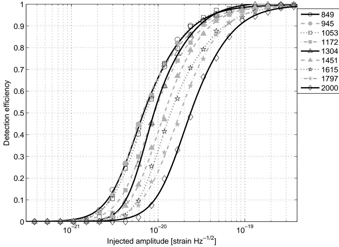
**Figure 5.** Detection efficiency of the WBCP pipeline for various sine-Gaussian simulated gravitational-wave bursts, as a function of the signal amplitude (defined by Eq. 18). The legend indicates the central frequency (Hz) of the injected signal.
