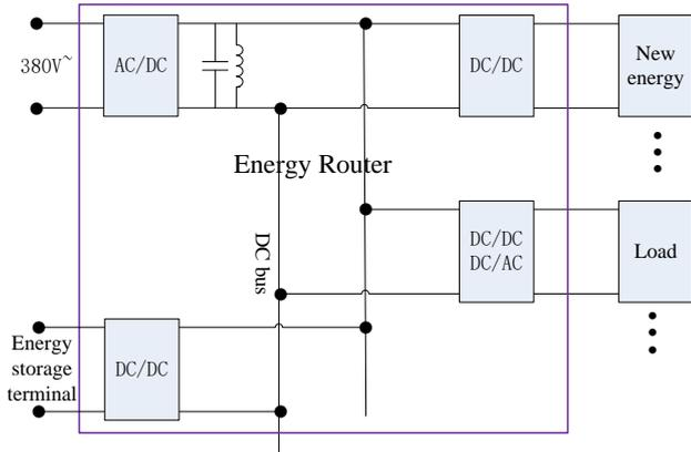
Fig. 1 Low-voltage ER structure
