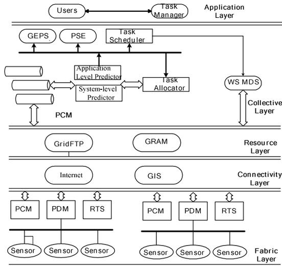
**Figure 1. Architecture of GHS performance evaluation and task scheduling system.**
