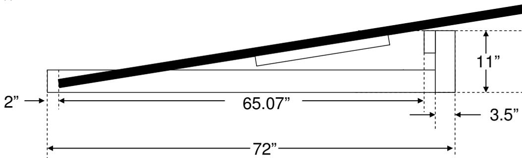
*Figure 5. Dimensions of the supine support structure*
