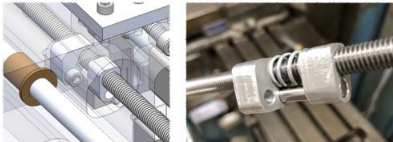
Figure 8: Overview of the anti-backlash system
