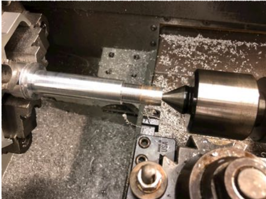
Figure 15: Single point threading of the spindle shaft
