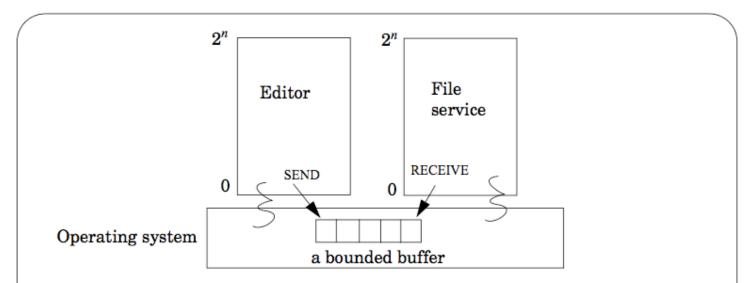
**Figure 5–2:** An operating system providing the editor and file service module each their own virtual computer. Each virtual computer has a thread that virtualizes the processor. Each virtual computer has a virtual address space that provides each module with the illusion that it has its own memory. To allow communication between virtual computers, the operating system provides SEND, RECEIVE, and a bounded buffer of messages.
