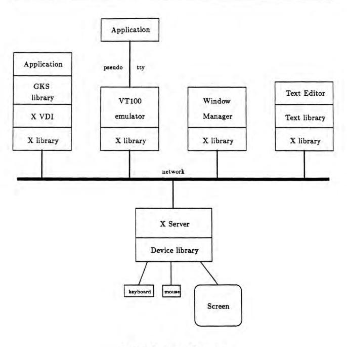
Figure 1: System Structure
