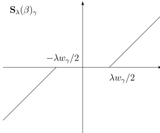
Figure 2: Thresholding function  $S_\lambda$  for iterative thresholding algorithm.
