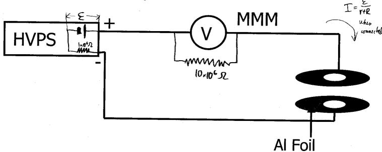
(a) What is the approximate reading of the multimeter in Volts when the EMF of the HVPS has been adjusted to 400V and the foil has not jumped?
