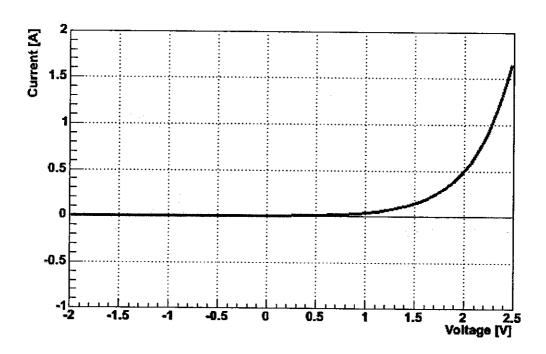
(a) Approximately, what is the resistance of the diode for an applied voltage of -2V?
