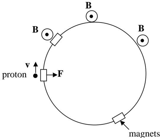
$\vec{F} = q\vec{v} \times \vec{B}$ . The direction of  $\vec{B}$  is shown in figure above.
